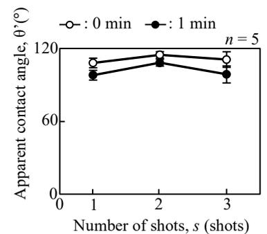
**Fig. 5** Measured results of the time-course changes of apparent contact angles by using FL processing.
