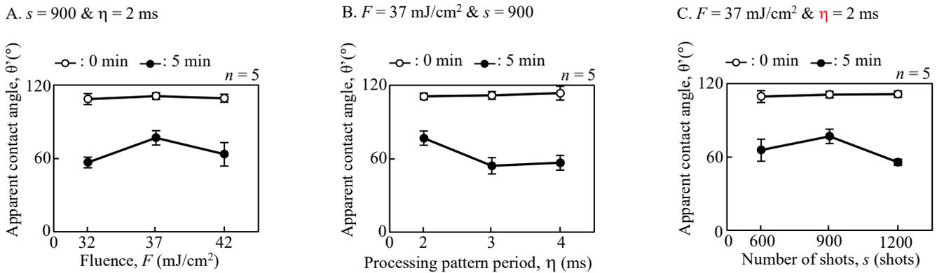
**Fig. 6** Measured results of the time-course changes of apparent contact angles by using PL processing.
