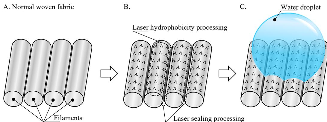
**Fig. 1** Proof-of-concept of ultrashort-pulsed laser modification for improving hydrophobicity as a physical approach.
