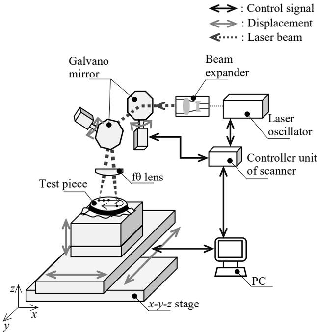
**Fig. 2** Configuration of ultrashort-pulsed laser systems used for direct processing on the surface of woven fabric of Nylon 6 (femtosecond-pulsed processing: with a beam expander, picosecond-pulsed processing: without a beam expander, PC: personal computer).
