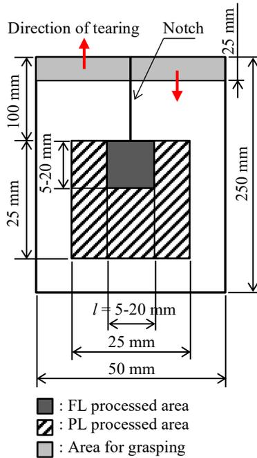
Fig. 4 Test-piece with both FL and PL processing for tearing test.
