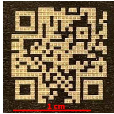
Fig. 8 Laser-processed sample: QR code printed onto anodized aluminum with pulsed IR laser via galvanometric scanner.
