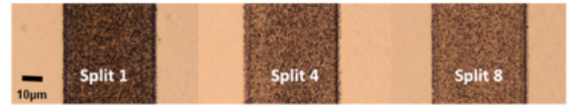
Fig. 11 Microscope images for a fixed feed speed and average power of 12W. Improved optical quality visible for higher amount of splitting.
