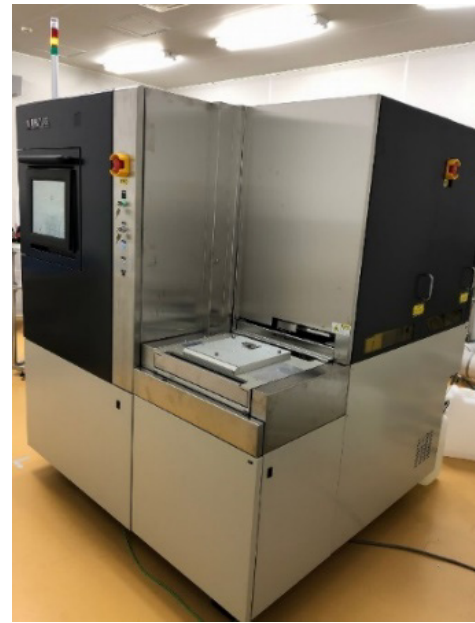
Fig. 5 DISCO fully automated laser dicing platform DFL7262.
